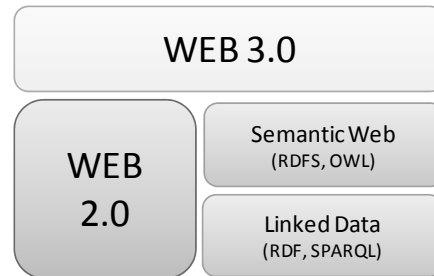
Fig. 4. Web 3.0 applications are Web 2.0 applications based on linked data and web semantic technologies
