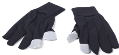
Fig. 2. Gloves with 4 points reflector that placed on fingers
